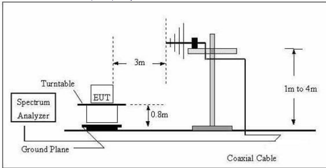
The radiated emission test were performed in the 3 meters chamber test site, using the setup accordance with the ANSI C63.10-2013. The specification used was the FCC 15.209 and FCC 15.205 limit.
