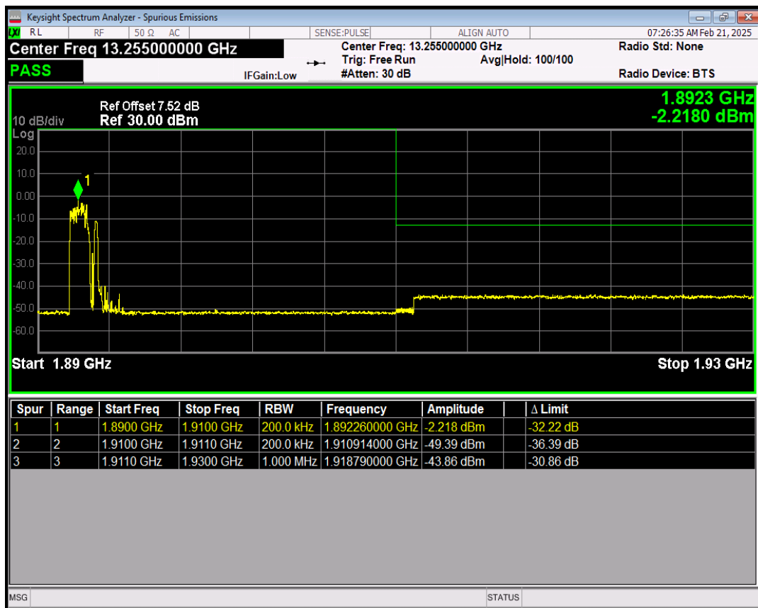
Band2 16QAM BW=20MHz Channel=19100 RB Size=1 Position=#Max
