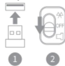
2. Slide the mouse power switch downward to 2.4G mode for instant use.
