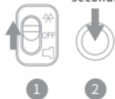
Press the Bluetooth button for at least 3 seconds to enter pairing mode.
