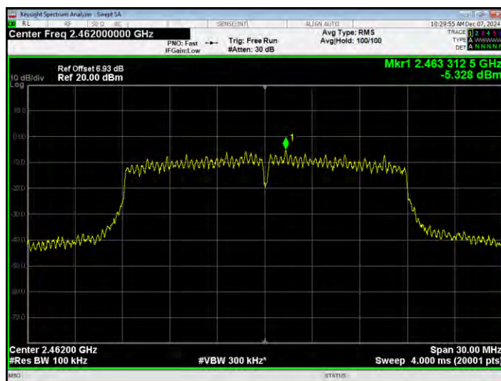
PSD NVNT n40 2422MHz Ant1
