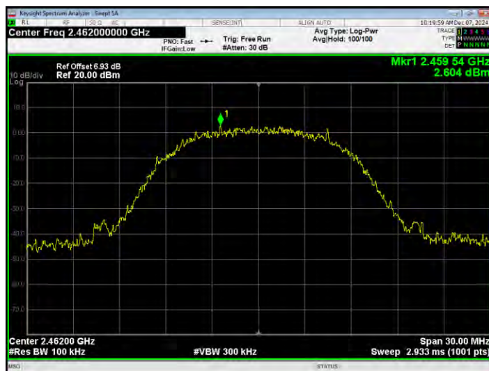
Band Edge NVNT b 2462MHz Ant1 Emission
