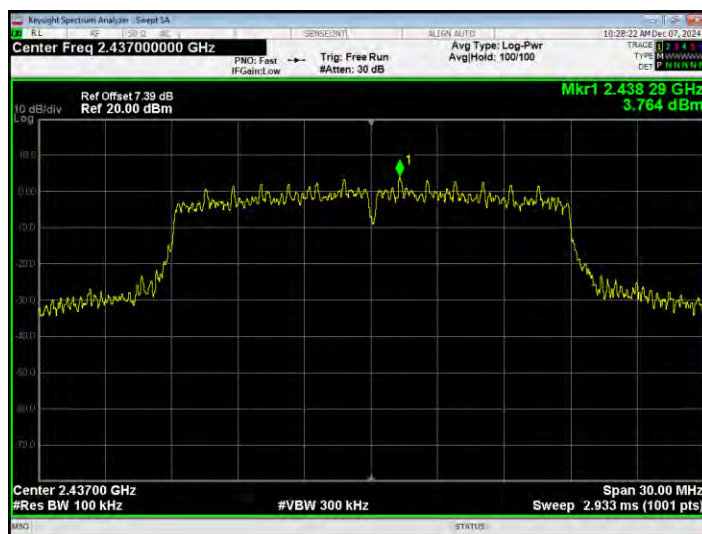
Tx. Spurious NVNT n20 2437MHz Ant1 Emission
