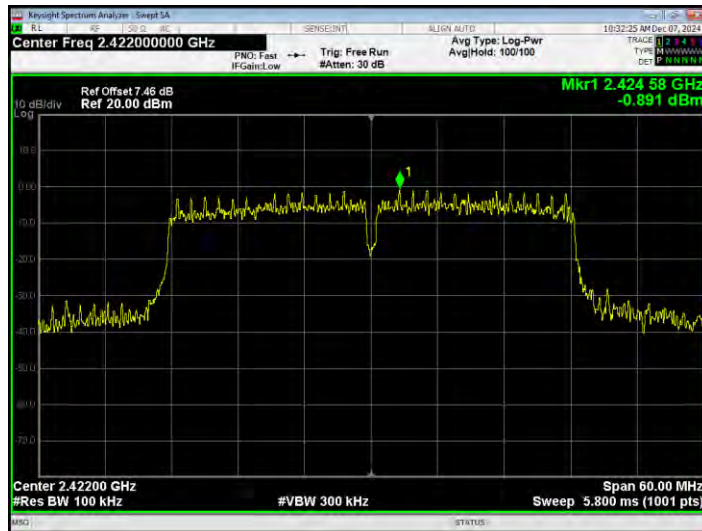
Tx. Spurious NVNT n40 2422MHz Ant1 Emission
