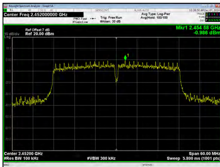
Band Edge NVNT n40 2452MHz Ant1 Emission
