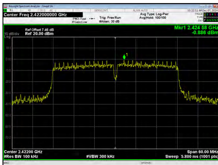
Band Edge NVNT n40 2422MHz Ant1 Emission
