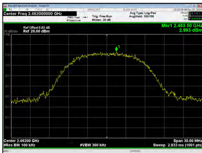
Tx. Spurious NVNT b 2462MHz Ant1 Emission
