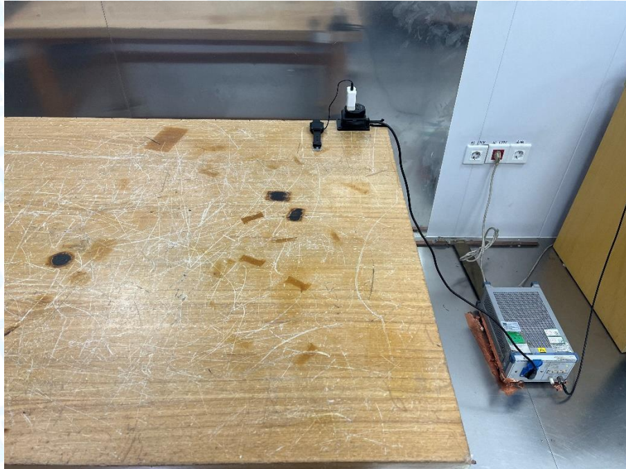
Photo of Setup for Radiated Emission (30MHz~1GHz)
