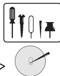
Use a tool (such as Sim card pin, mini screw driver, fine needle as above) to press the elastic button meanwhile push the battery cover down
