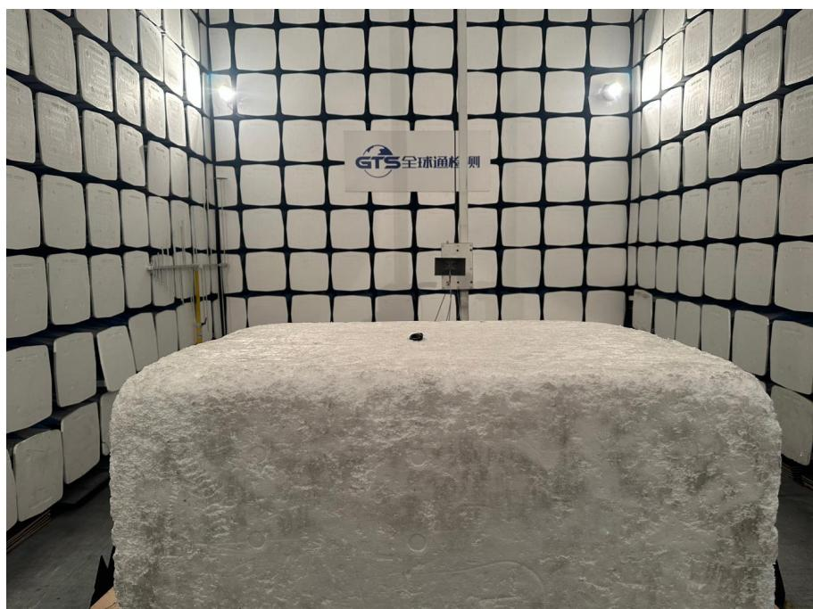
1.2 .Photo of Conducted Emission Measurement
