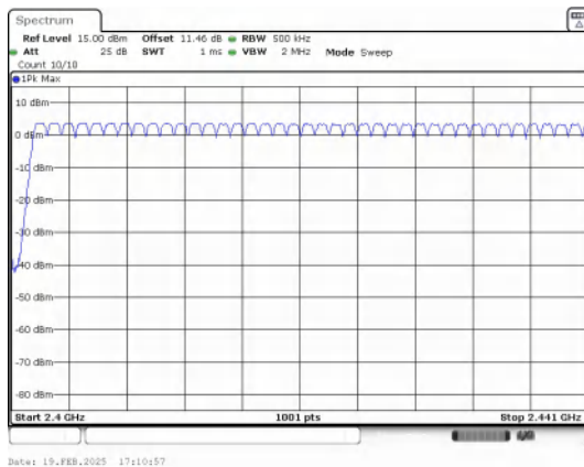
Low End Spectrum Channel Hopping Plot GFSK
