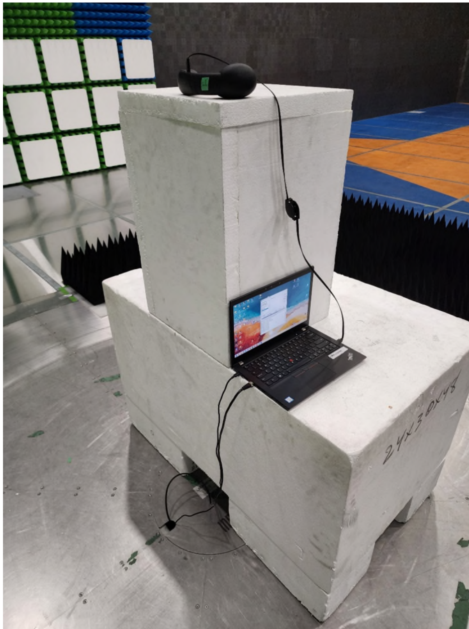
Figure 3 – Radiated Emissions Setup
