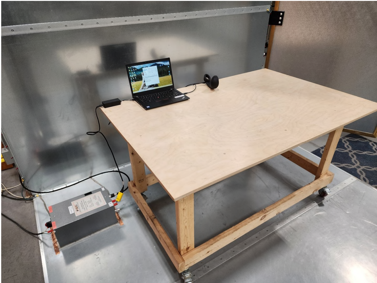
Figure 9 – Power Line Conducted Emissions Setup
