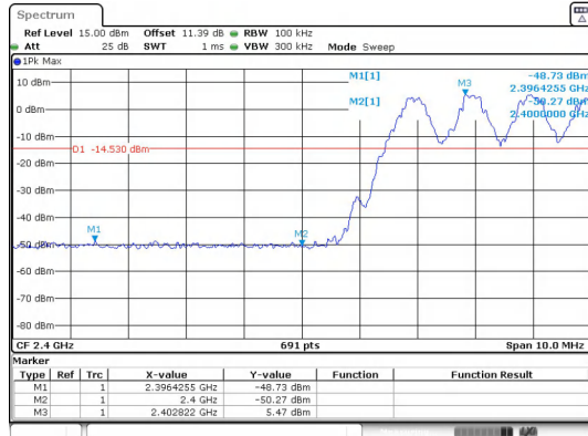
Out Of Band Emission(Left) GFSK_DH5_Channel Hopping
