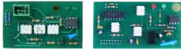
Nuovo Pignone interface boards for RS-485 interface for monoproduct and multiproduct dispensers
