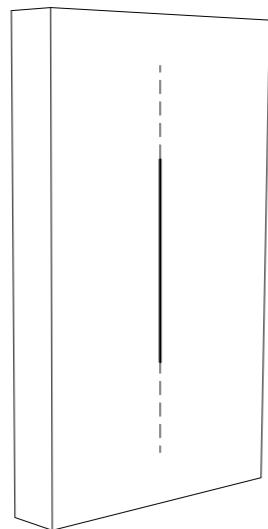
3. Place the wall dock with the center holes aligned with the vertical line. Mark the four lower mounting holes (A) and remove the wall dock.
