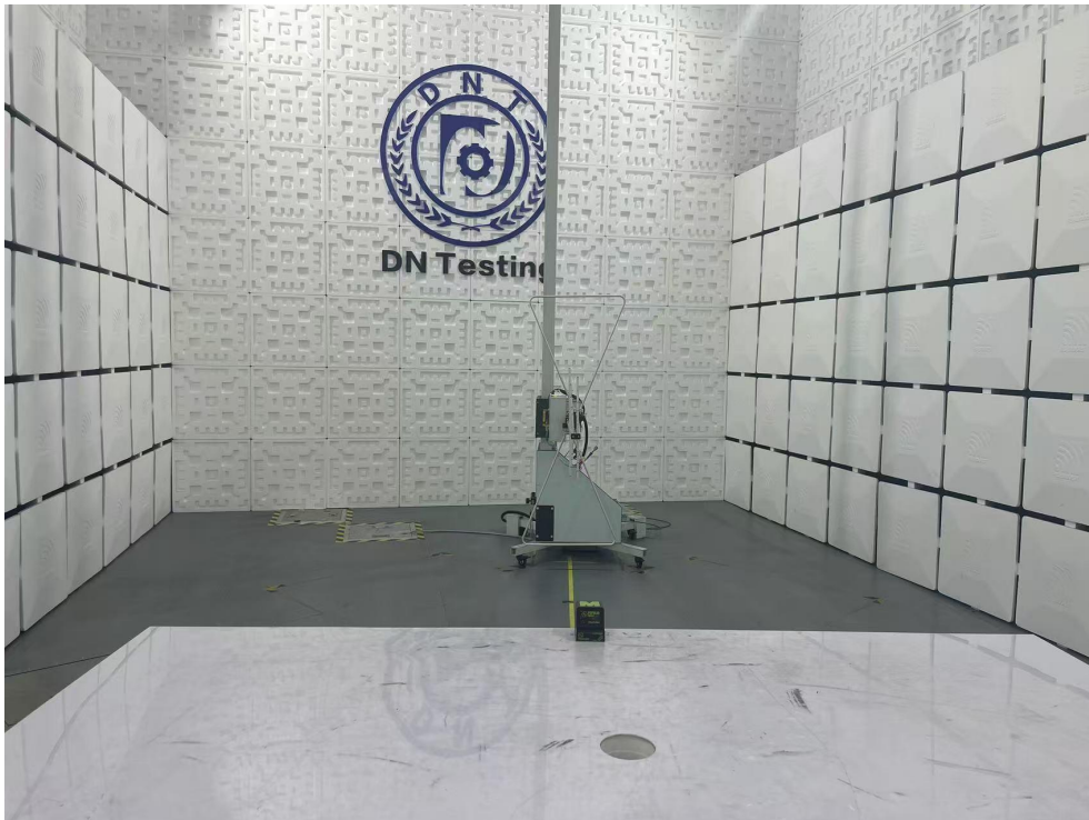
Radiated Emission Test View|(Below 1G)
