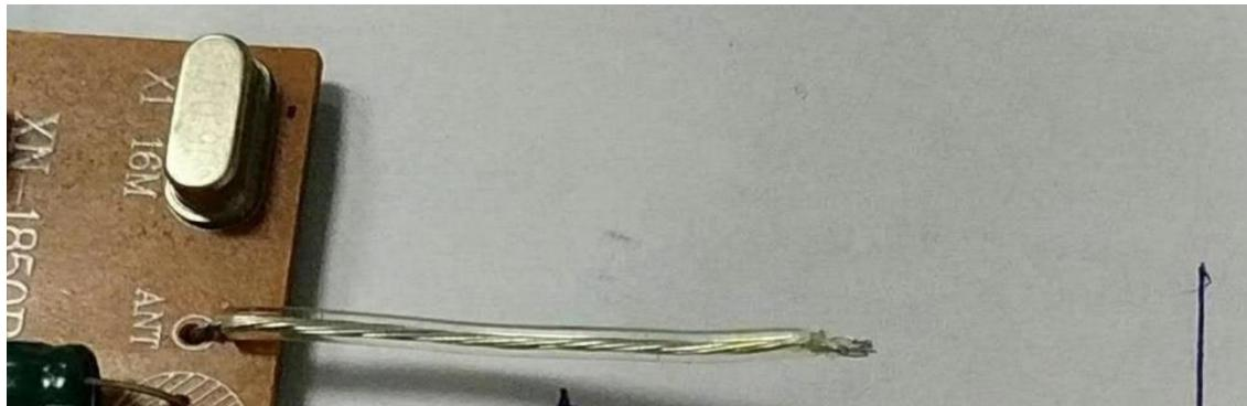
Note: 2.4G antenna specifications are 19-core outer diameter 1.38MM tinned copper wire, transparent color, length of 35MM, wire tip peeled 3MM tin. In line with environmental standards: EU EN71(19E), ROHS, PAHS, 6P~ 16P, European and American CPSIA, HR4040.
