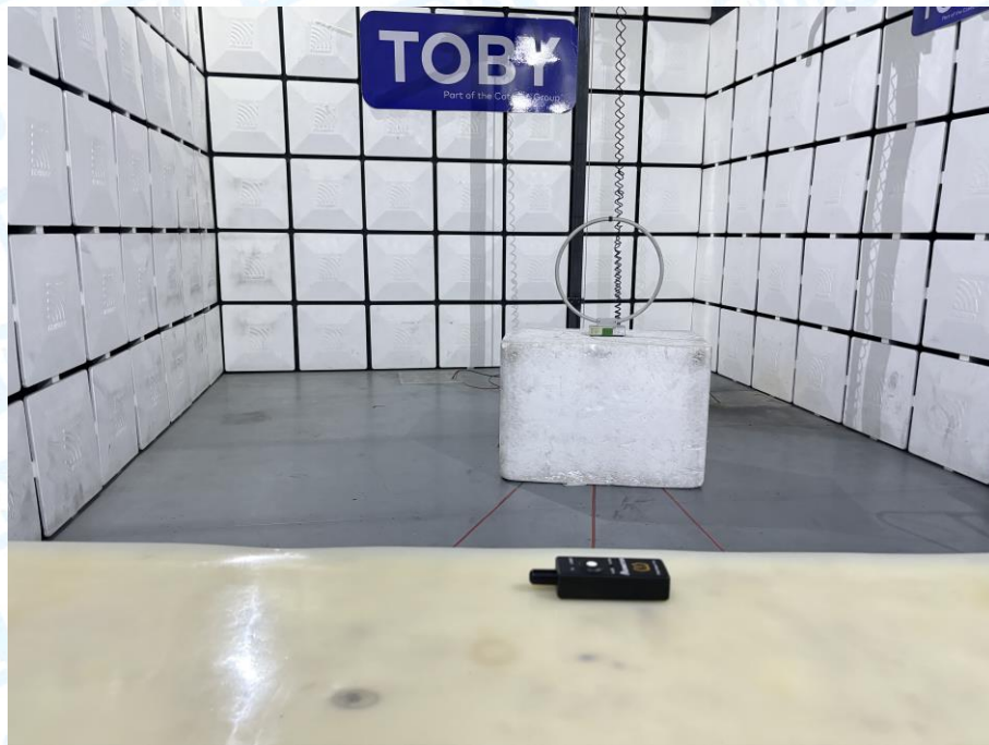
Photo of Setup for Radiated Emission (Below 30 MHz)
