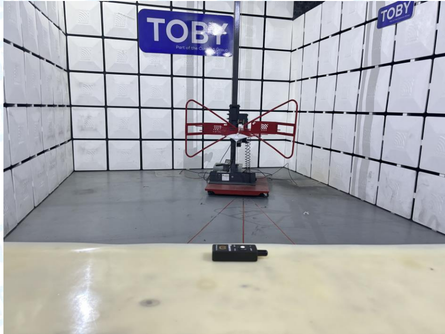
Photo of Setup for Radiated Emission (Below 30 MHz)
