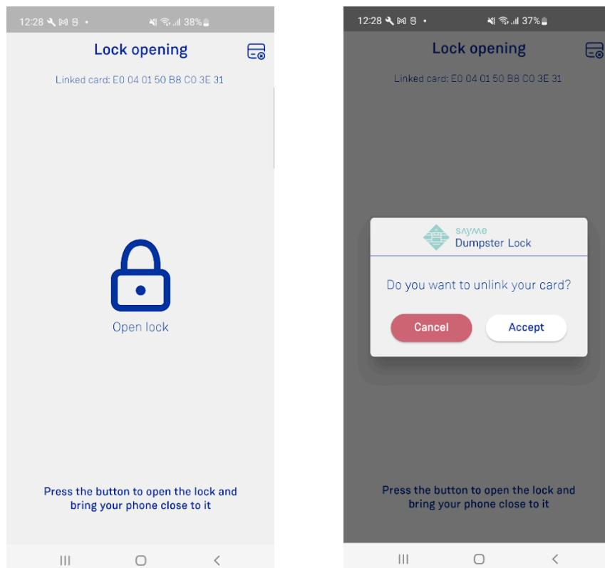
Once linked, the user can press the "Open Lock" button in the app and bring the phone close to the lock's reader. From this point, the process is the same as with the NFC card:
