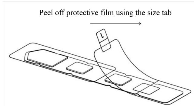
Figure 8 Peeling off the Electrode Band protective film
