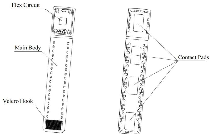
Figure 3. Schematic diagram of the Connector Band
