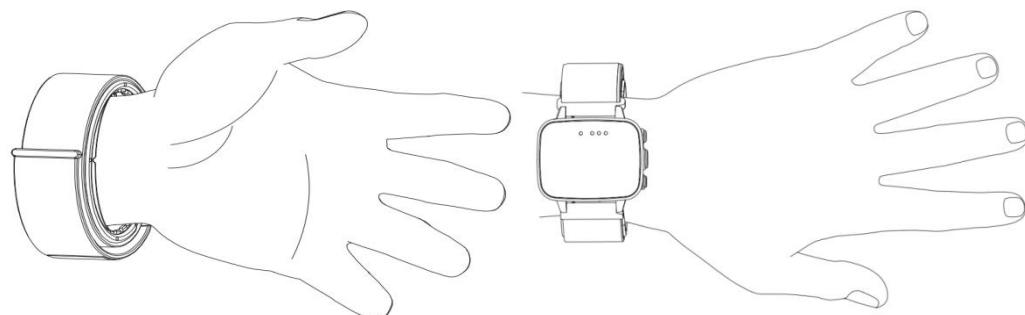
Figure 9 Align white dots on the Connector Band with the notches of the Electrode Band
