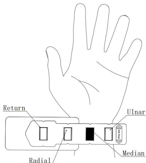
Figure 7 Schematic diagram of the Electrode Band placement
