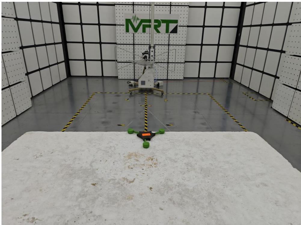
Description: Radiated Emissions Test Setup for 1GHz ~ 18GHz
