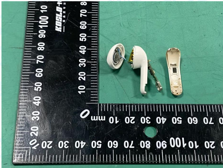
Photo 22 Appearance of PCB & Battery---L
