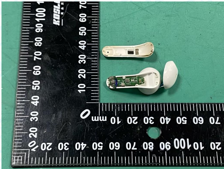
Photo 16 Internal of Battery---R
