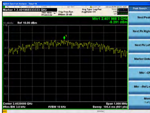
GFSK (BLE 1Mbps) LOW CHANNEL
