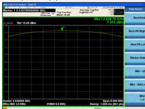
GFSK (BLE 2Mbps) MIDDLE CHANNEL
