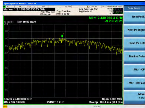
GFSK (BLE 1Mbps) MIDDLE CHANNEL
