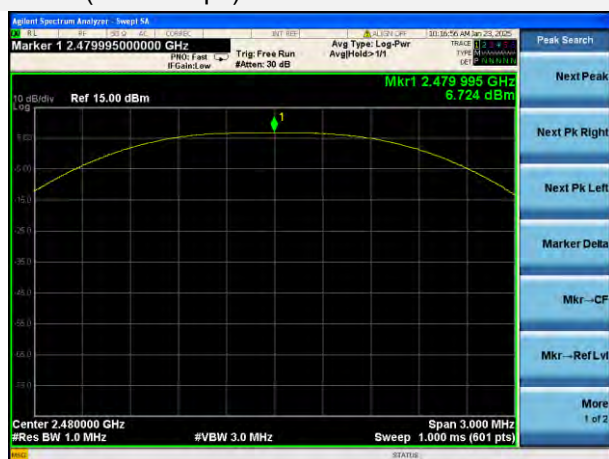
GFSK (BLE 1Mbps) HIGH CHANNEL
