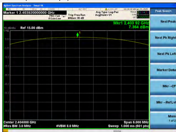
GFSK (BLE 2Mbps) LOW CHANNEL
