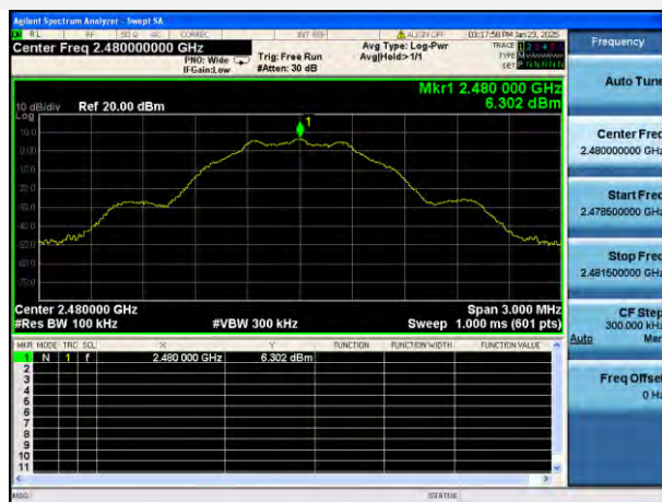
GFSK (BLE 1Mbps) HIGH CHANNEL, CARRIER LEVEL
