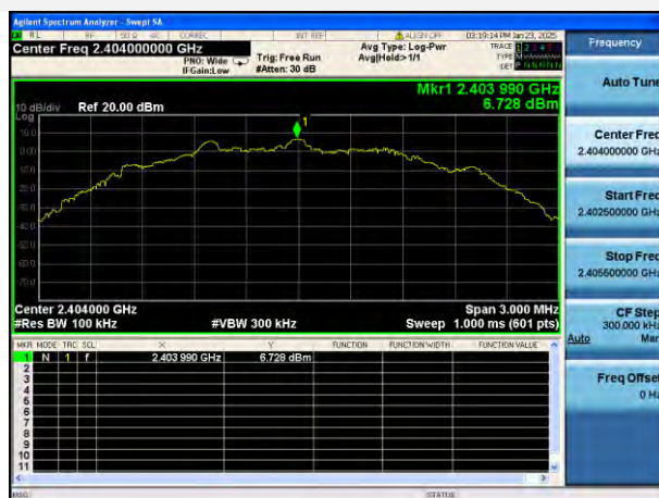
GFSK (BLE 2Mbps) LOW CHANNEL, CARRIER LEVEL
