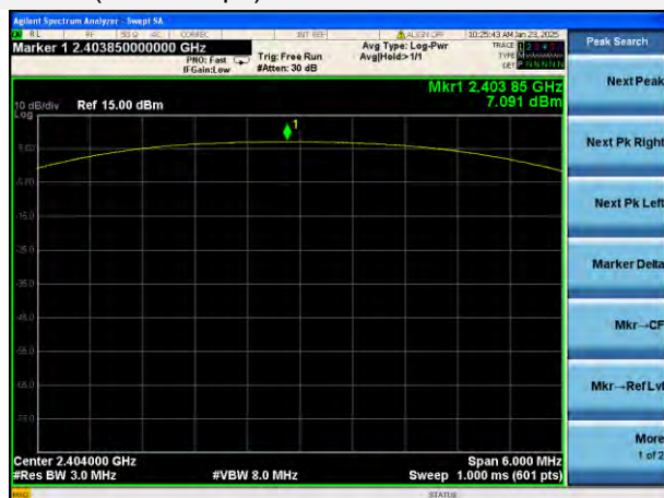
GFSK (BLE 2Mbps) LOW CHANNEL
