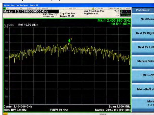
GFSK (BLE 2Mbps) LOW CHANNEL
