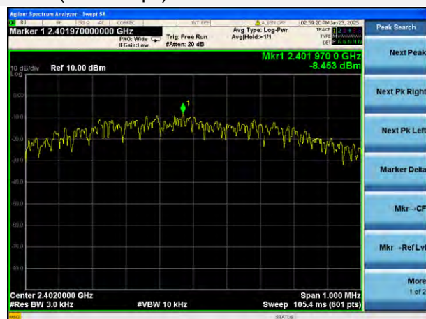
GFSK (BLE 1Mbps) LOW CHANNEL
