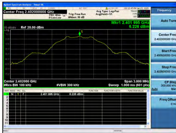
GFSK (BLE 1Mbps) LOW CHANNEL, CARRIER LEVEL
