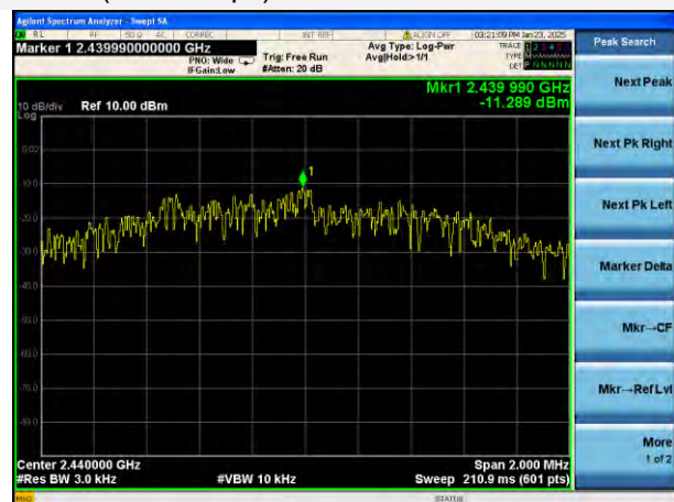
GFSK (BLE 2Mbps) MIDDLE CHANNEL
