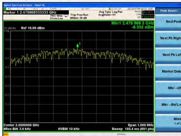
GFSK (BLE 1Mbps) HIGH CHANNEL
