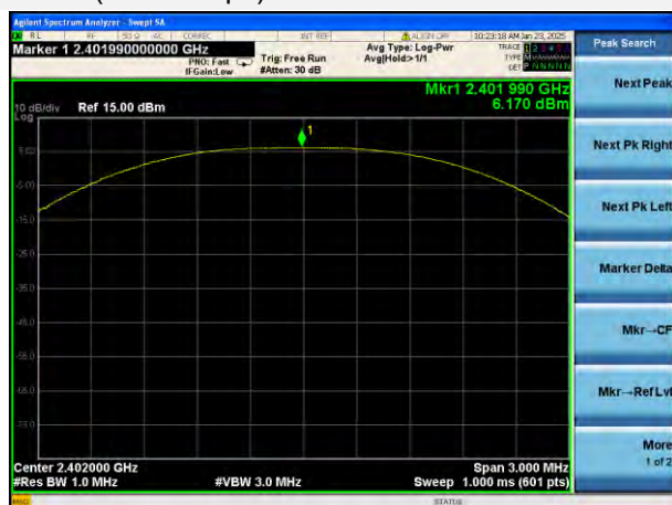
GFSK (BLE 1Mbps) LOW CHANNEL
