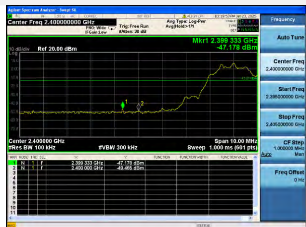
GFSK (BLE 2Mbps) LOW CHANNEL, BAND EDGE
