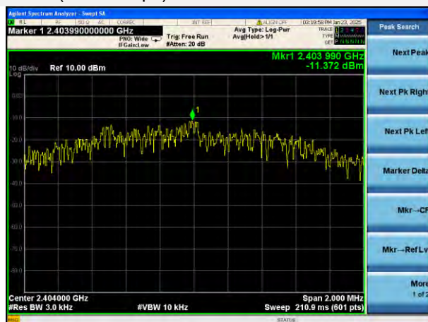
GFSK (BLE 2Mbps) LOW CHANNEL
