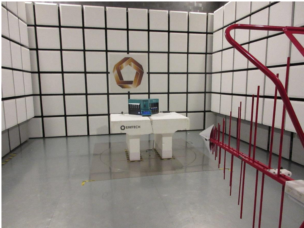
TEST SETUP PHOTO(S) - ANSI C63.4
