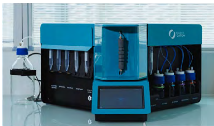
Figure 4.2: Instrument in process configuration with CTC-POD® which contains Seefer®
