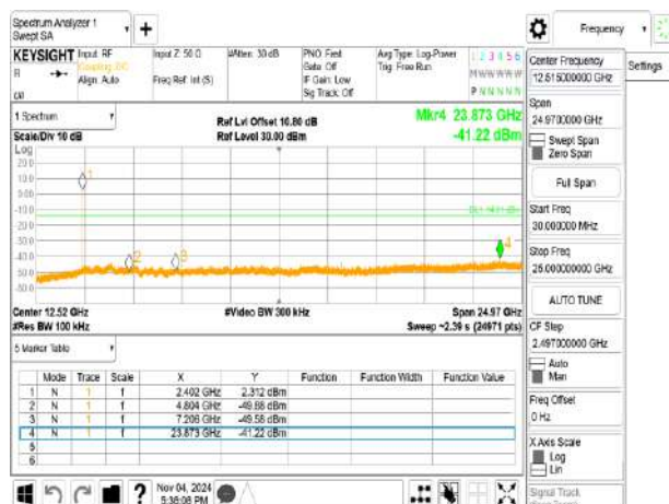
Spurious Emission_BLE 2M_LowCH00-2402MHz
