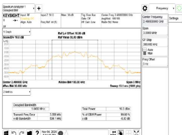
IC OBW_BLE 125k_HighCH39-2480MHz
