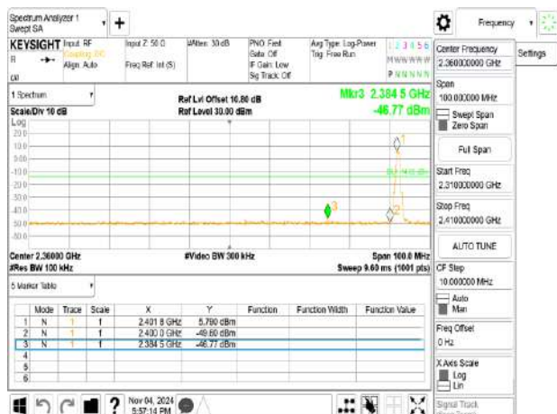
Band Edge_BLE 500k_HighCH39-2480MHz
