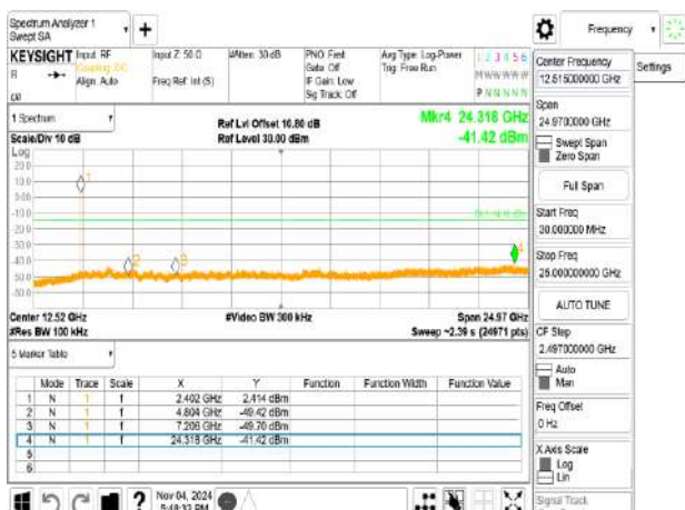
Spurious Emission_BLE 125k_LowCH00-2402MHz
