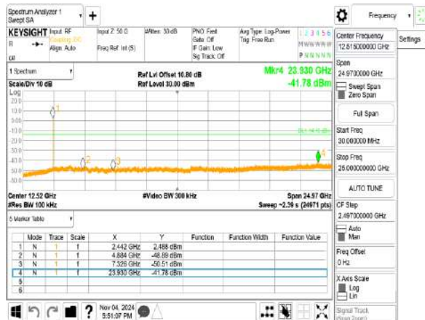
Spurious Emission_BLE 125k_HighCH39-2480MHz
