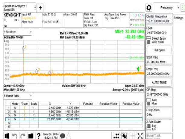
Spurious Emission_BLE 2M_LowCH00-2402MHz
