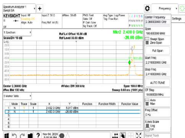
Band Edge_BLE 2M_LowCH00-2402MHz
