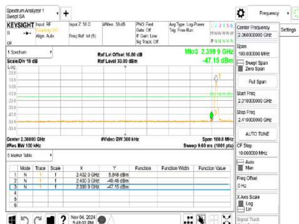
Band Edge_BLE 125k_HighCH39-2480MHz
