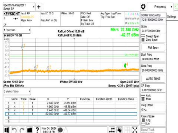
Spurious Emission_BLE 500k_LowCH00-2402MHz
