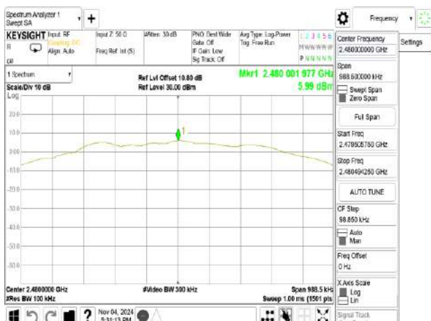
Reference Level_BLE 1M_HighCH39-2480MHz
