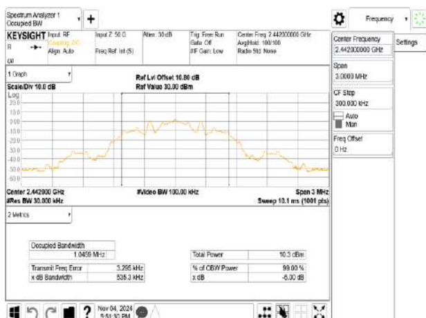
IC OBW_BLE 125k_HighCH39-2480MHz
