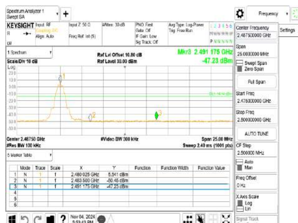
Band Edge_BLE 125k_HighCH39-2480MHz
