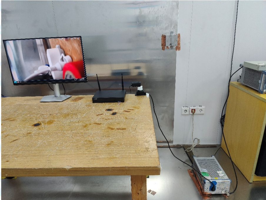
Photo of Setup for Radiated Emission (30MHz~1GHz)
