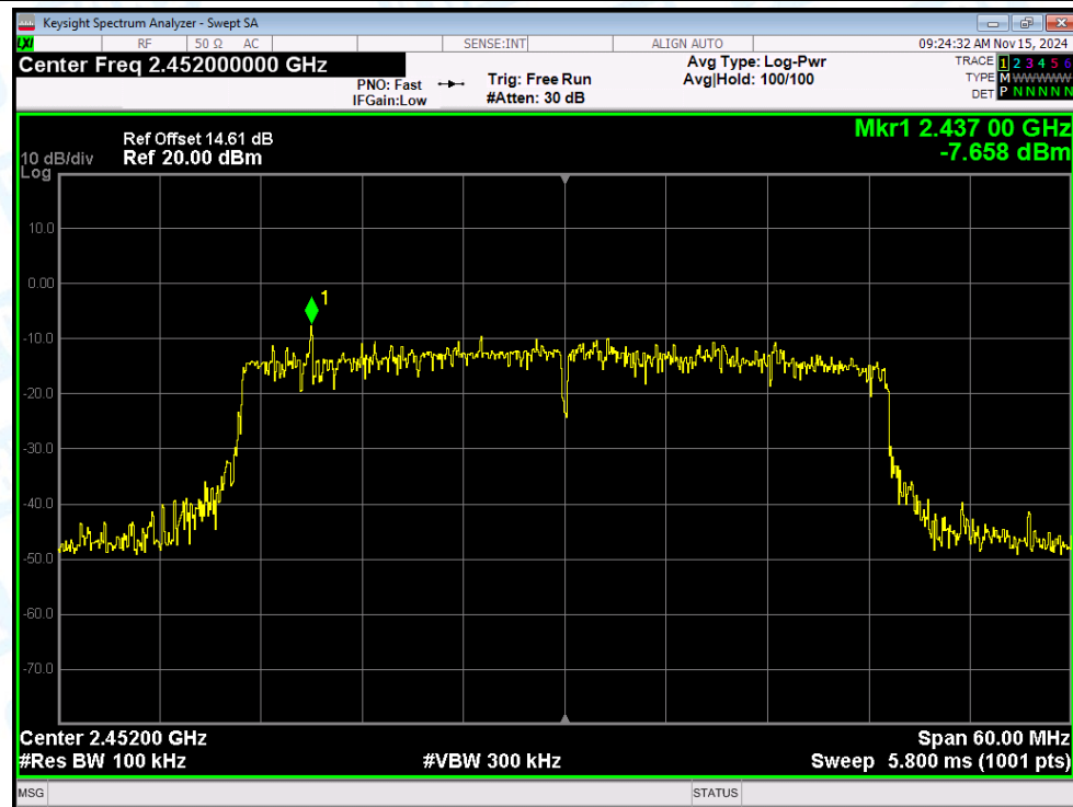
Band Edge NVNT ax(VHT40) 2452MHz Ant1 Emission
