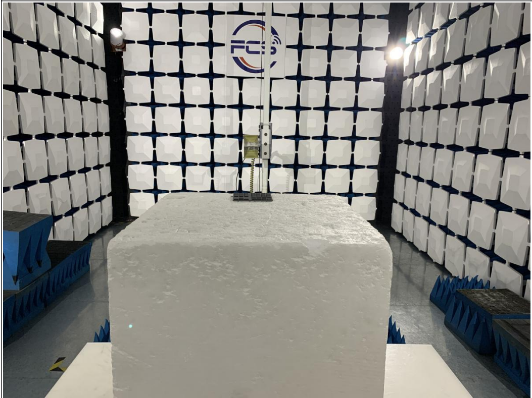
Above 1GHz for radiated emission test setup
