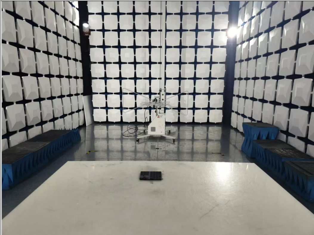
Above 1GHz for radiated emission test setup
