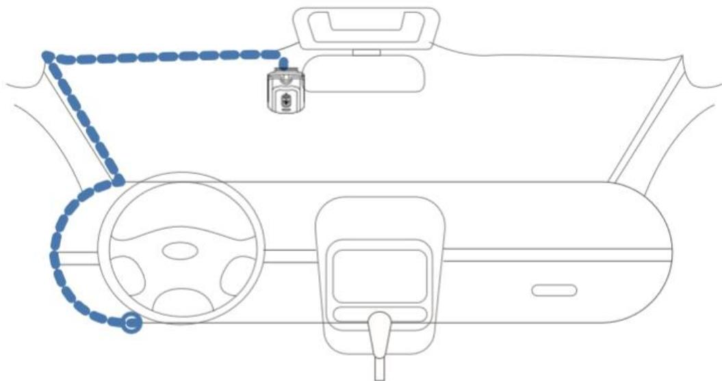
Through the safe box can facilitate the driving recorder to take power, can make it work safely, but also make the recorder line more hidden, the car cloth safe box location: most models of the safe box location in the left side of the driving position or near the steering wheel. Refer to the car instructions for details.
