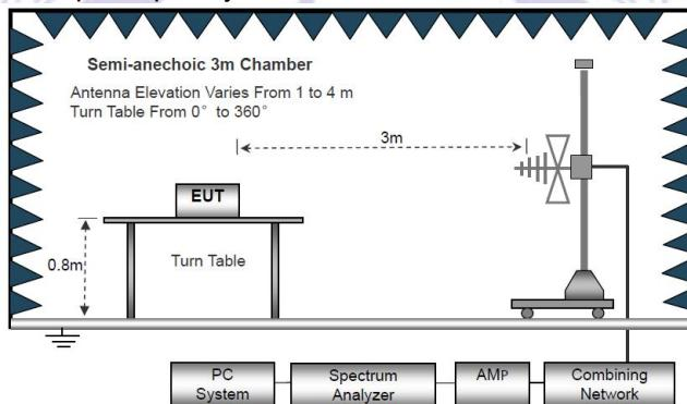
(C) Radiated Emission Test-Up Frequency Above 1GHz
