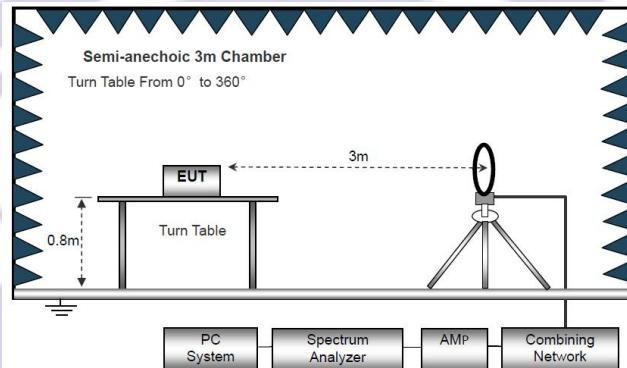
(B) Radiated Emission Test-Up Frequency 30MHz~1GHz
