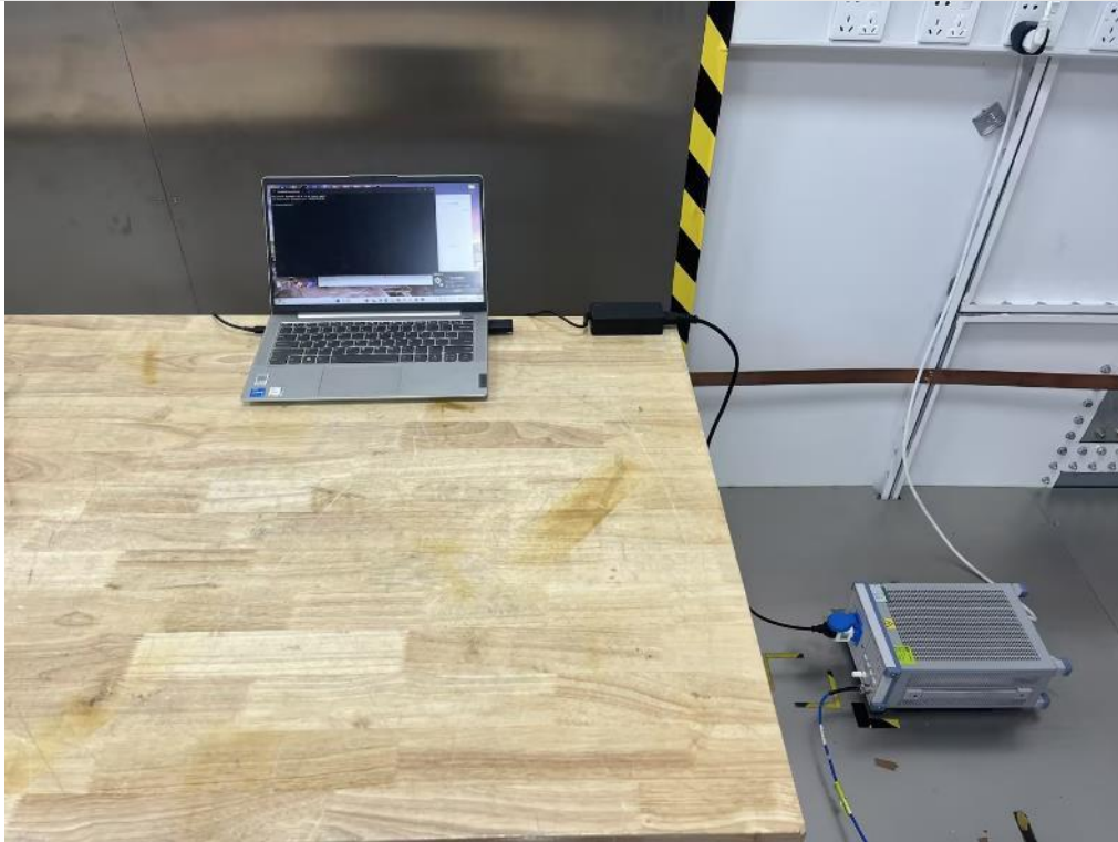
AC Power Line Conducted Emission
