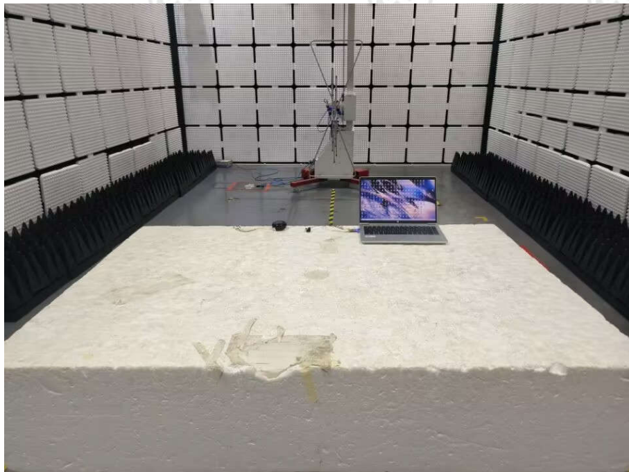
Radiated spurious emission Test Setup-2 Ear R (Below 1GHz)
