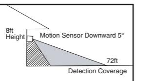
When mounted 8ft above the ground and the sensor is 5° down, the maximum sensing distance is about 72ft.
