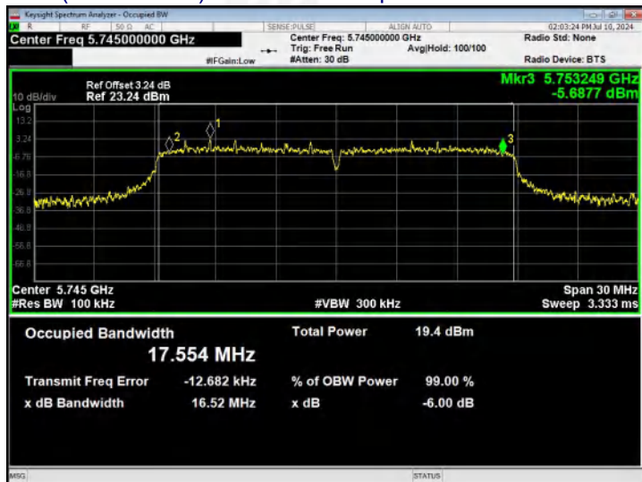
(802.11 ac20) 6dB Bandwidth plot on channel 157
