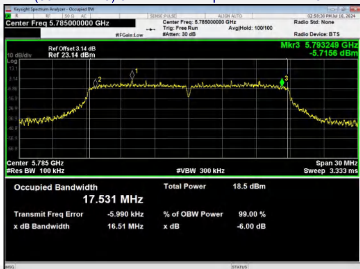
(802.11 ac20) 6dB Bandwidth plot on channel 165
