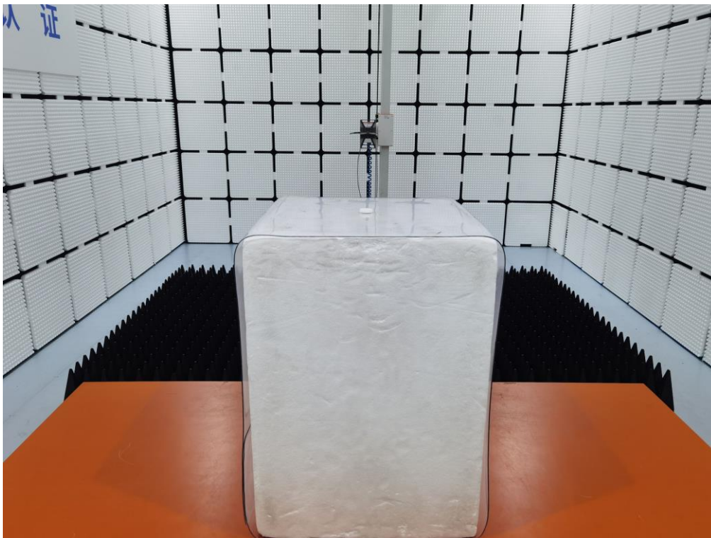
Radiated Emission Above 1GHz
