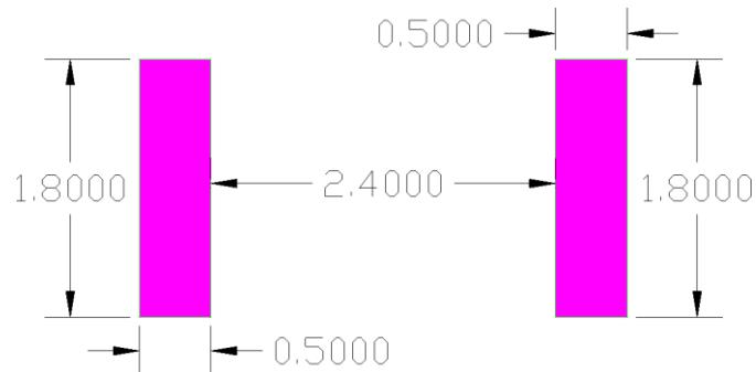
◆ 2<sup>nd</sup> Layout Dimensions in Clearance area( size=8.0\*3.0mm)
