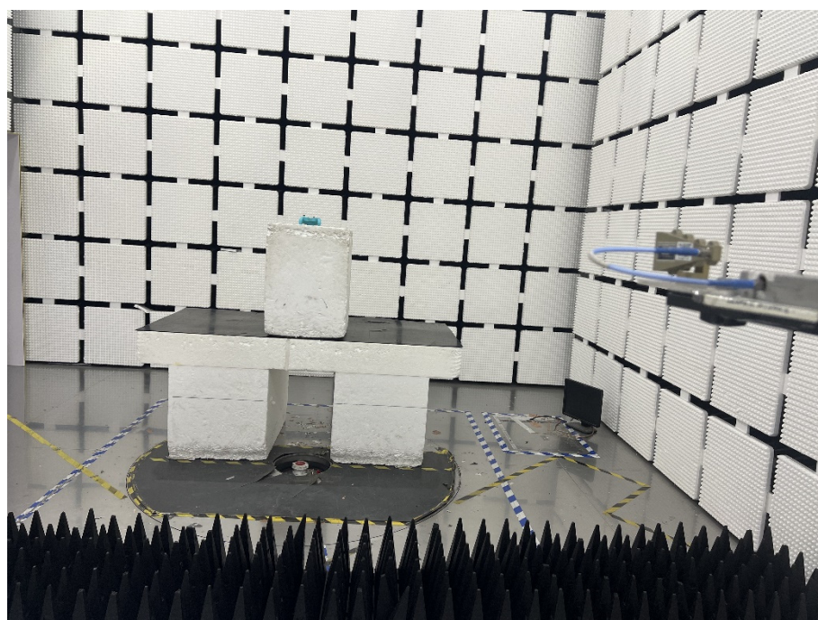
Radiation Emission Test Setup (Above 18GHz)
