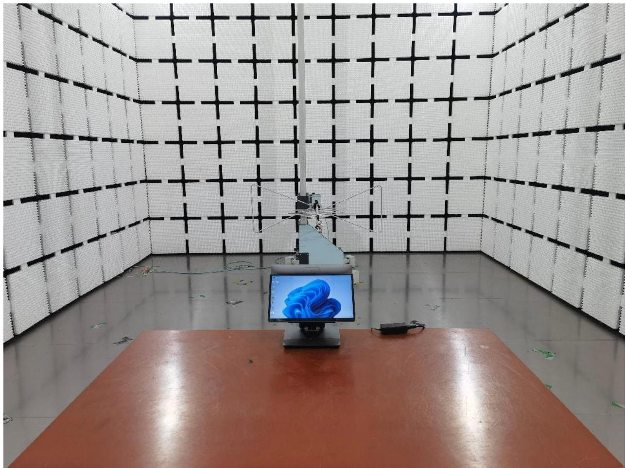
**Radiated Emission Test View 2**
