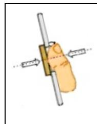
Place your finger firmly on the sensor and align the core of the fingerprint to the center of the sensor. The sensor will scan your fingerprint automatically.
