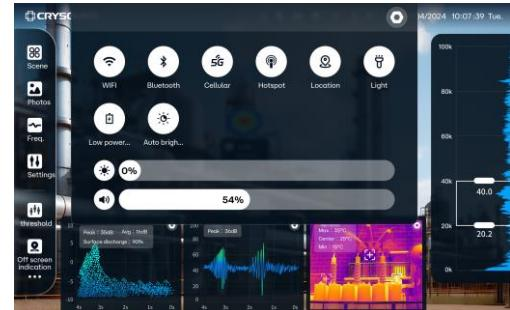
Long pressing the thermal image enters the dragging mode, allowing you to drag the thermal image to the upper area of the main screen to display it in the thermal view. Dragging the thermal image to the left or right area enters the split-screen display mode.
