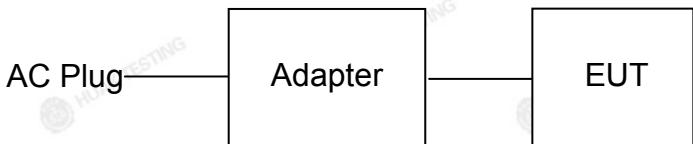
Operation of EUT during above 1GHz Radiation testing:
