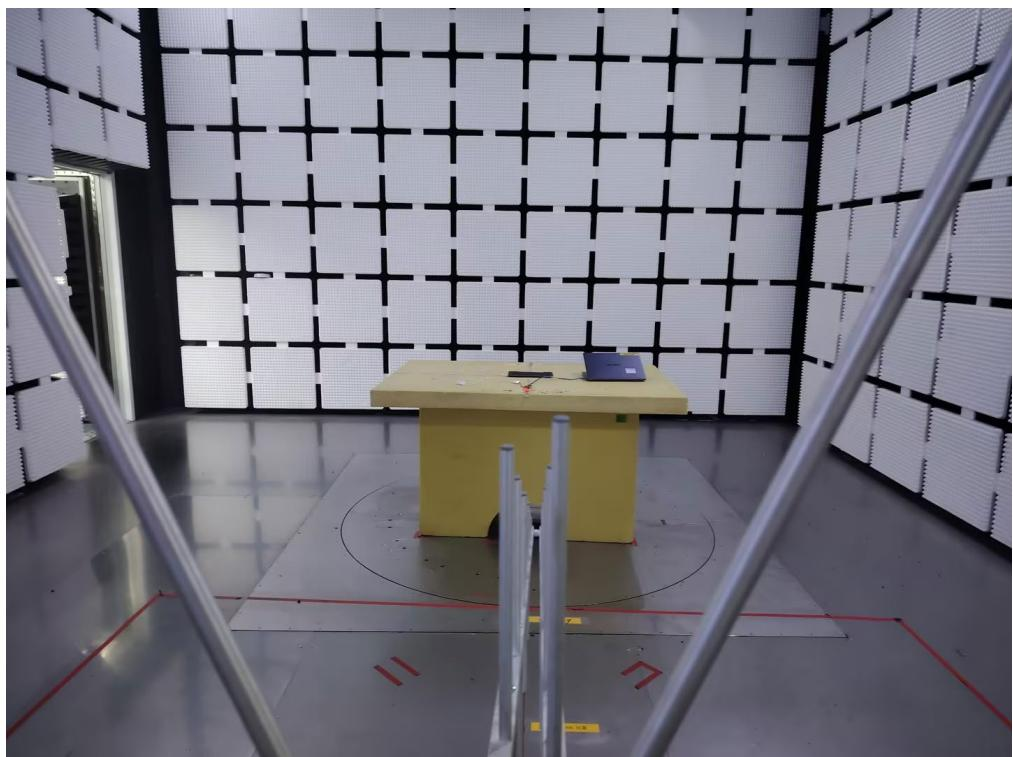
**Radiated Emissions Test Photos****1 GHz to 18 GHz**
