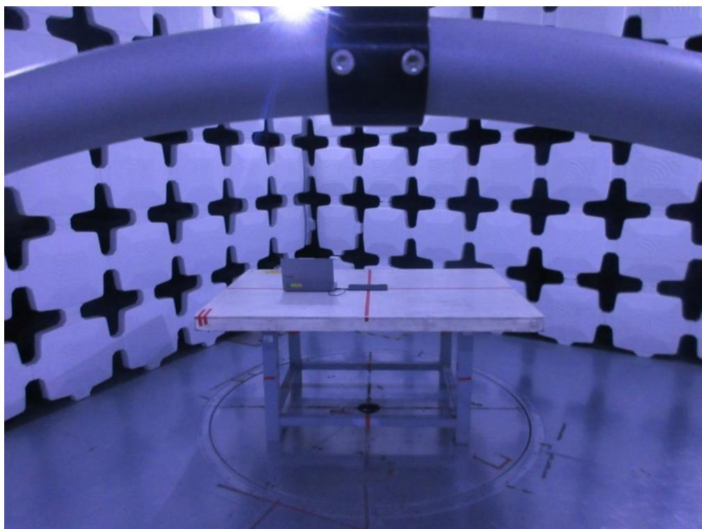
**Radiated Emissions Test Photos****30 MHz to 1000 MHz**
