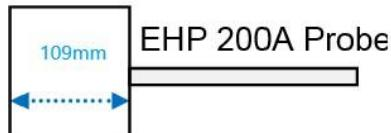
Notes: The EHP 200A Probe has a diameter of 10.9cm and a radius of 5.45cm.
