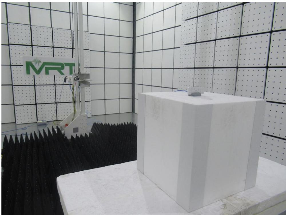
Description: Radiated Spurious Emission Test Setup for 18 ~ 25GHz
