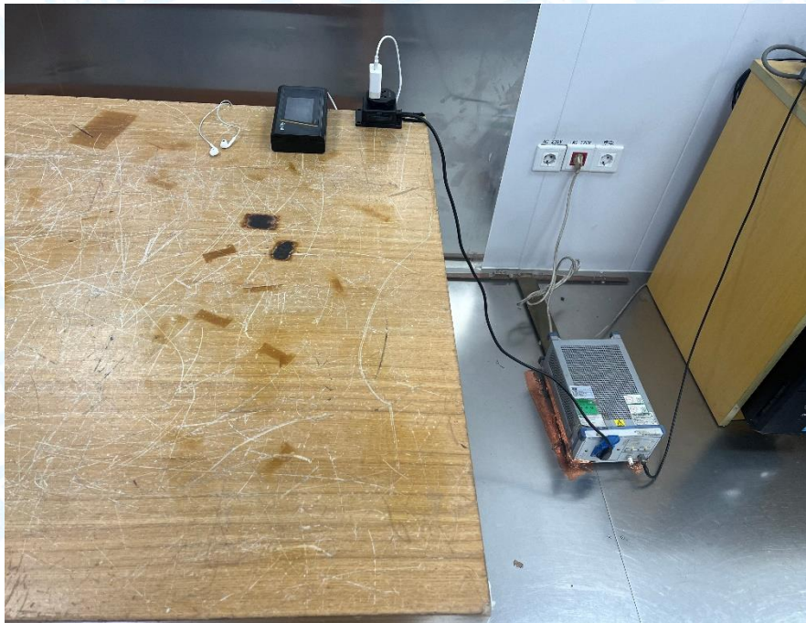
Photo of Setup for Conducted Emission
