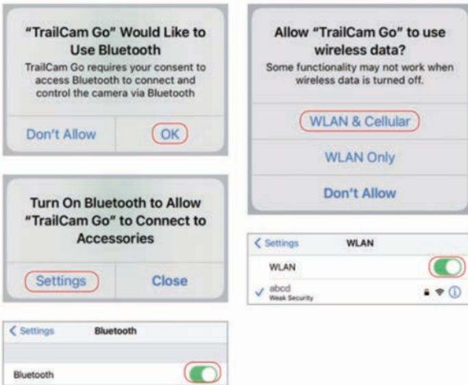
2. Ensure your camera is in "TEST" or "ON" mode. For a stable connection, please stay within 16 meters (55 feet) of your camera.
