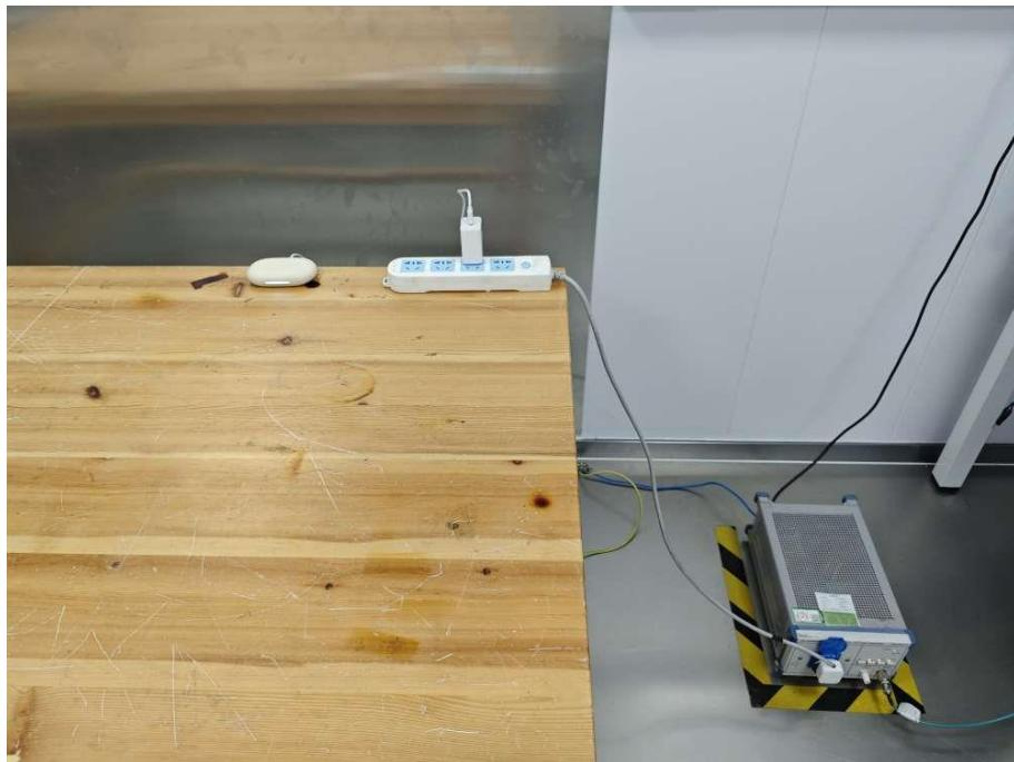
**Radiated Emission Test View Below 1GHz (Left earphone)**
