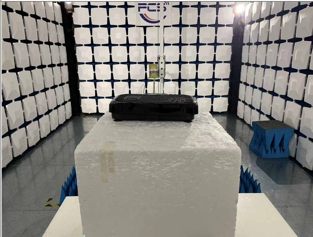
Above 1GHz for radiated emission test setup
