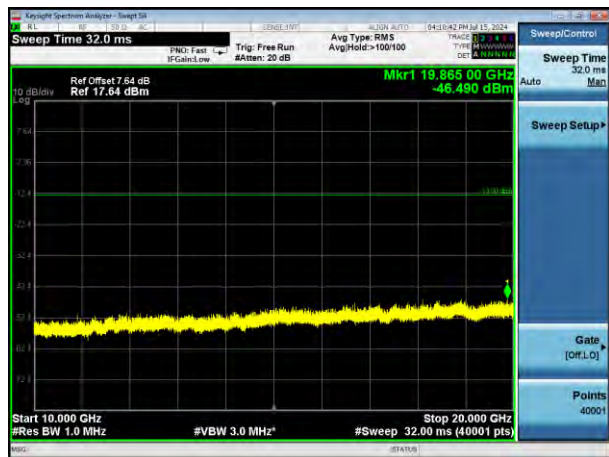
Band4 QPSK BW=10MHz Channel=20000 RB Size=50 Position=#0
