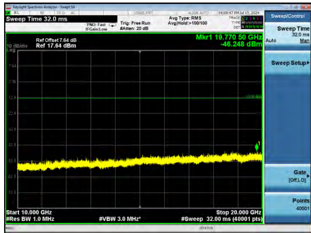
Band4 QPSK BW=3MHz Channel=20385 RB Size=15 Position=#0
