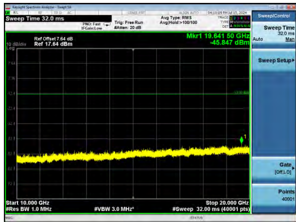
Band4 QPSK BW=5MHz Channel=20375 RB Size=25 Position=#0
