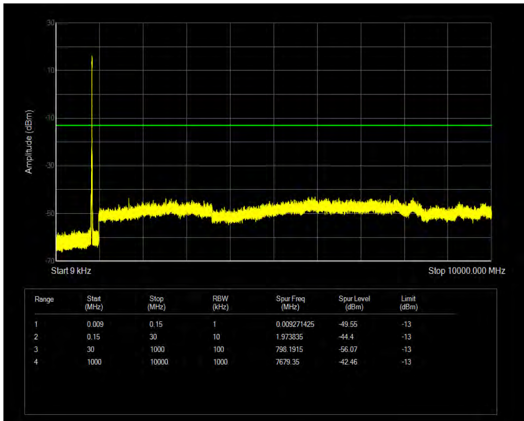
Band5 QAM16 BW=5MHz Channel=20625 RB Size=25 Position=#0
