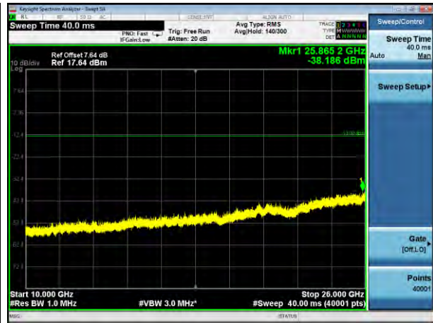
Band7 QAM16 BW=10MHz Channel=20800 RB Size=50 Position=#0
