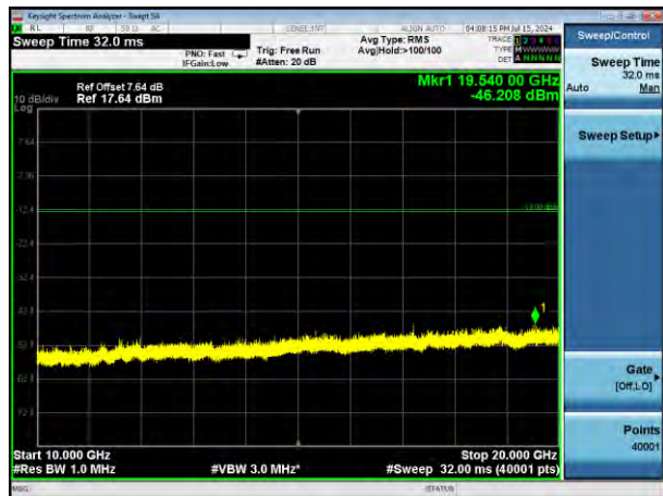
Band2 QAM16 BW=3MHz Channel=18615 RB Size=15 Position=#0
