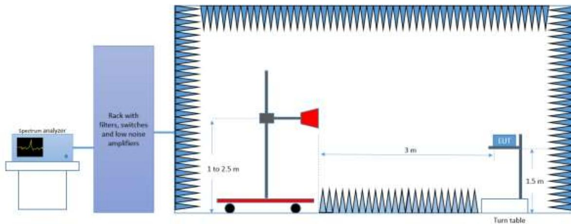
*Radiated Setup 6.4 GHz – 18 GHz*
