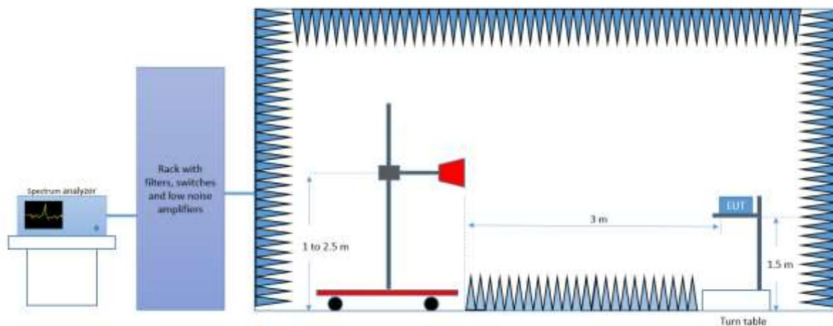
*Radiated Setup 18 GHz – 26.5 GHz*
