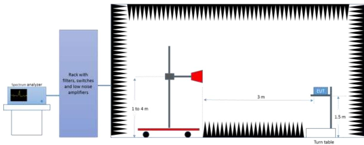
*Radiated Setup 6.4 GHz – 18 GHz*
