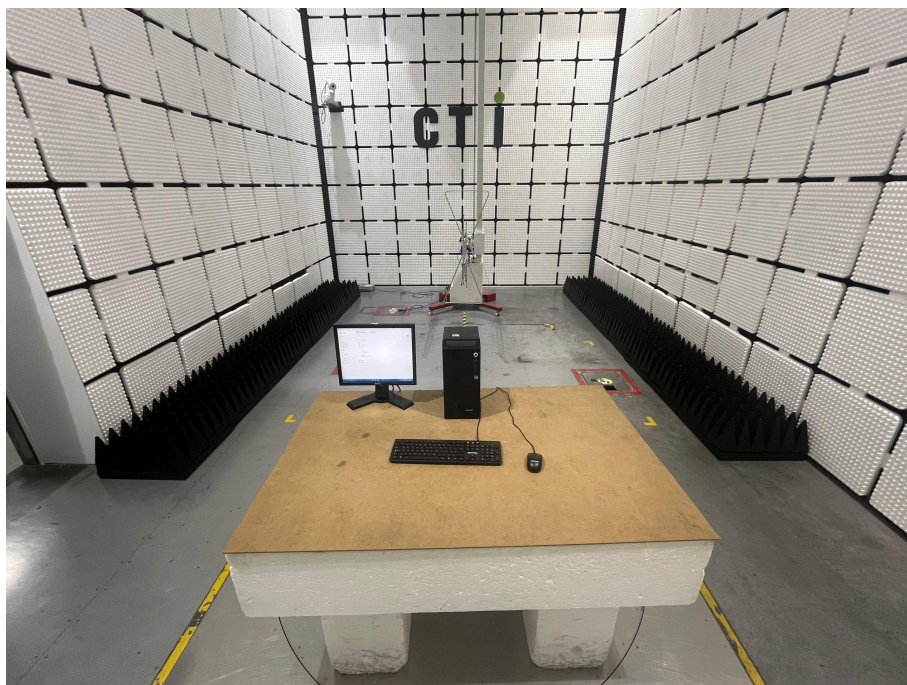
Radiated spurious emission Test Setup-1(Below 1GHz)
