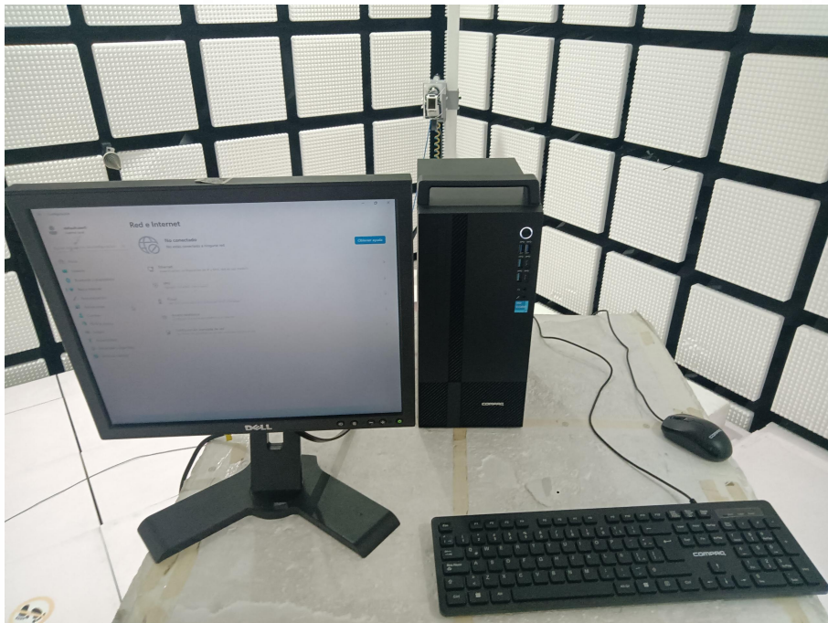
Radiated spurious emission Test Setup-3(Above 18GHz)
