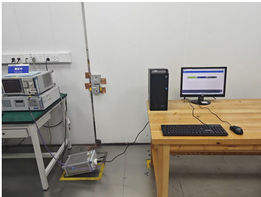
Conducted Emissions Test Setup
