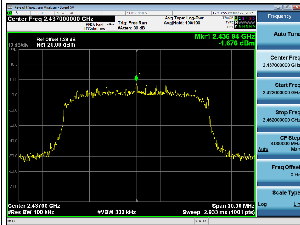
Tx. Spurious NVNT n20 2437MHz Ant1 Emission
