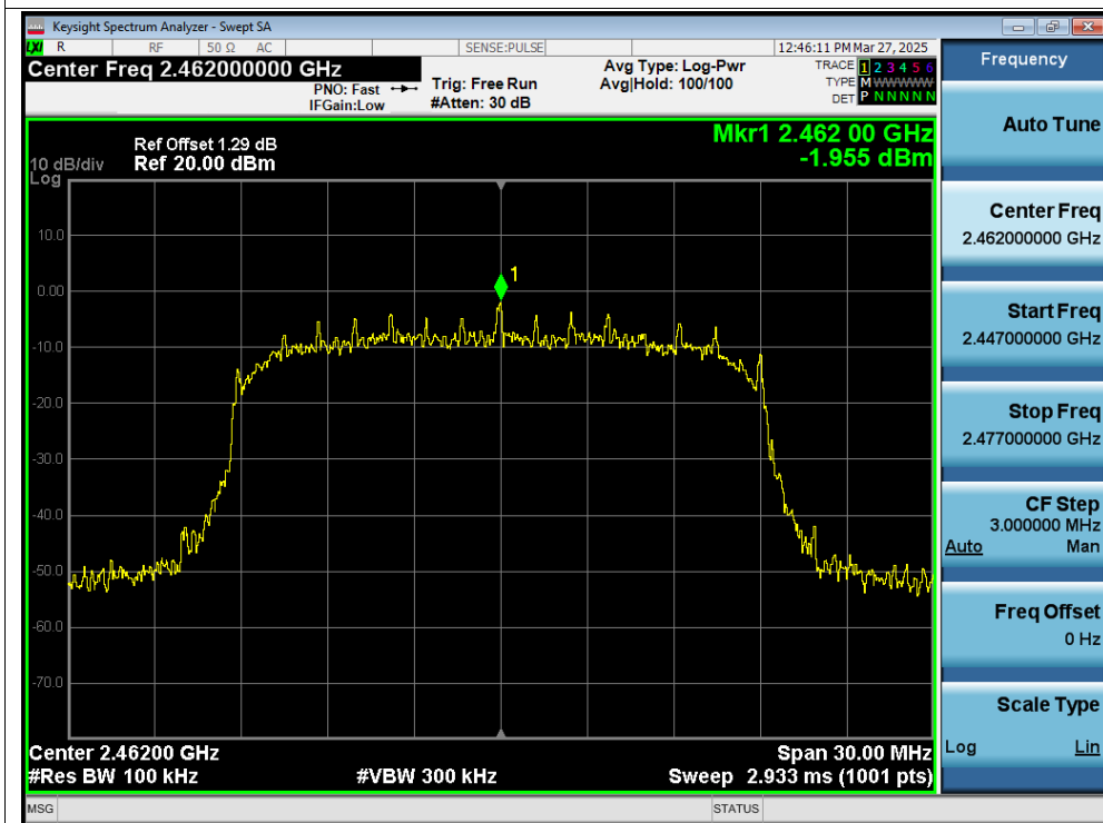
Band Edge NVNT n20 2462MHz Ant1 Emission
