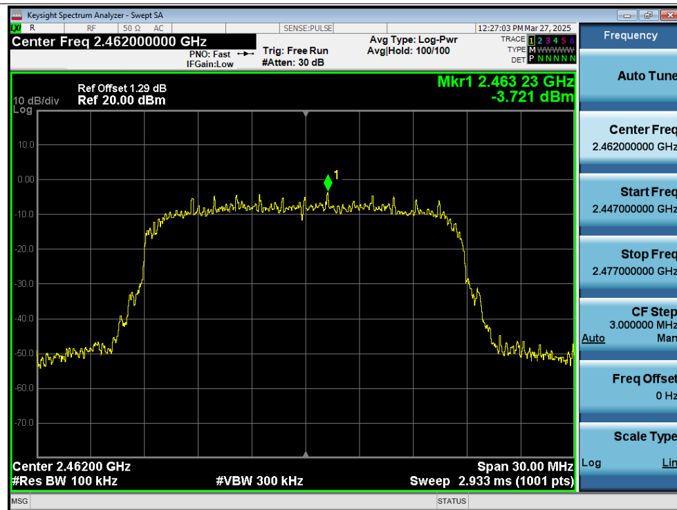
Band Edge NVNT g 2462MHz Ant1 Emission
