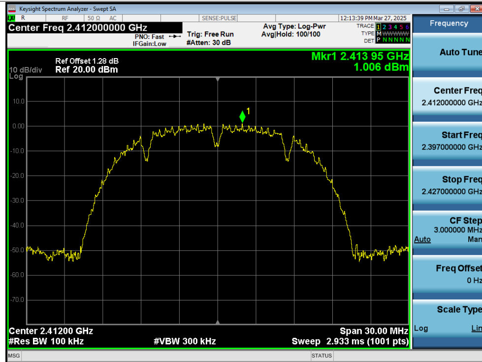
Band Edge NVNT b 2412MHz Ant1 Emission
