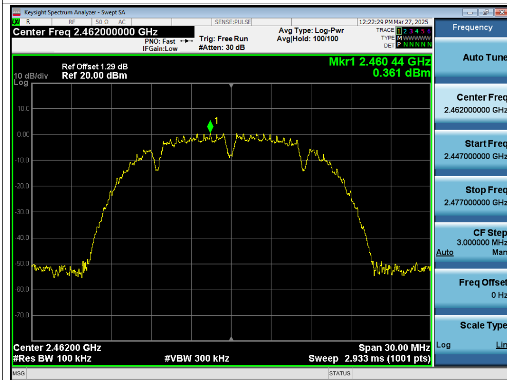
Tx. Spurious NVNT b 2462MHz Ant1 Emission
