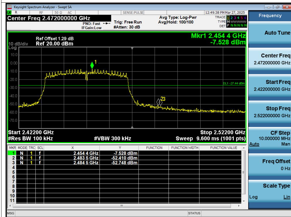
Band Edge NVNT n40 2452MHz Ant1 Emission
