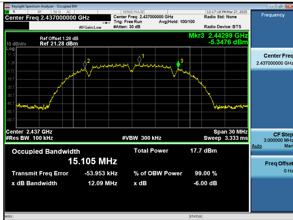
-6dB Bandwidth NVNT b 2437MHz Ant1
