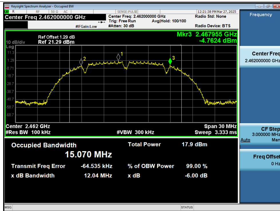
-6dB Bandwidth NVNT g 2412MHz Ant1
