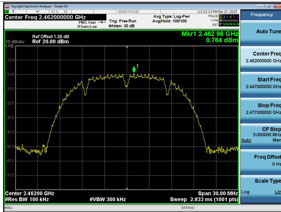
Band Edge NVNT b 2462MHz Ant1 Emission
