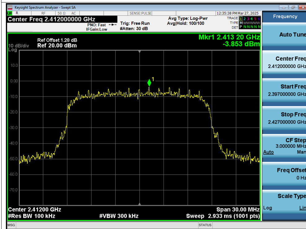
Tx. Spurious NVNT g 2412MHz Ant1 Emission
