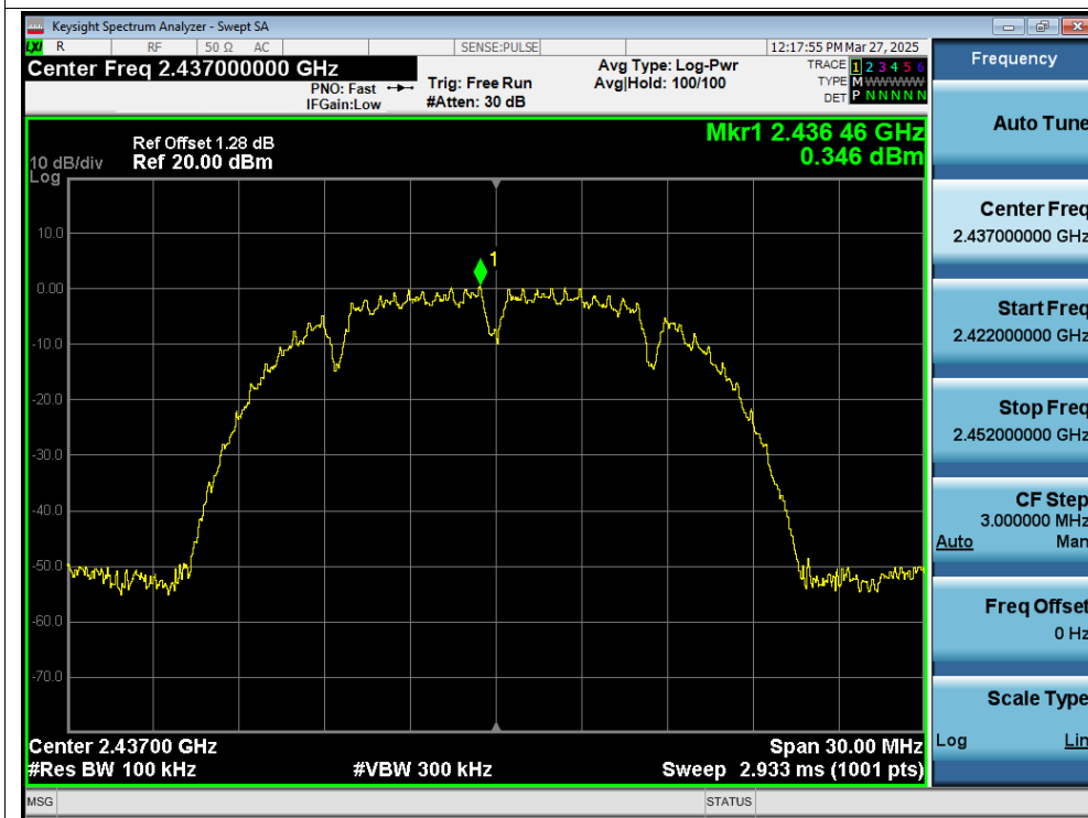
Tx. Spurious NVNT b 2437MHz Ant1 Emission
