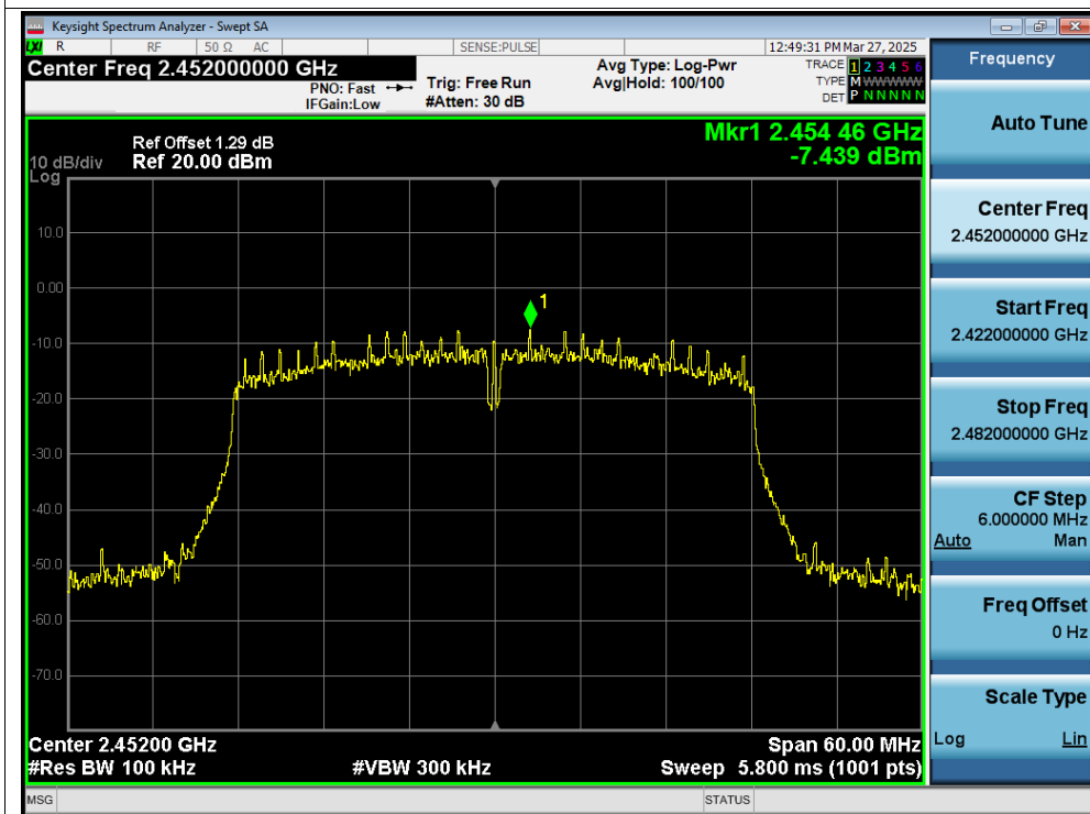
Band Edge NVNT n40 2452MHz Ant1 Emission
