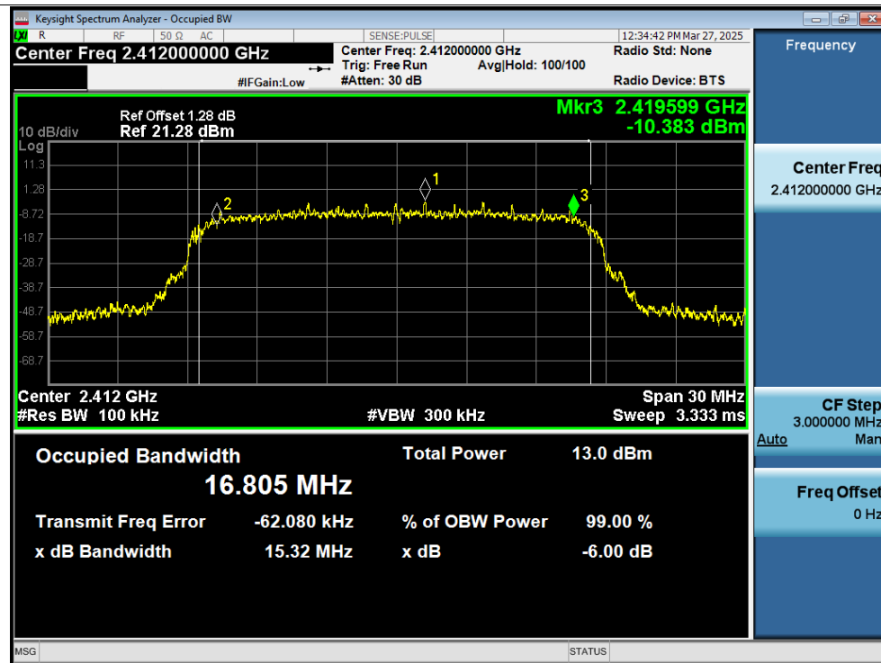
-6dB Bandwidth NVNT g 2412MHz Ant1
