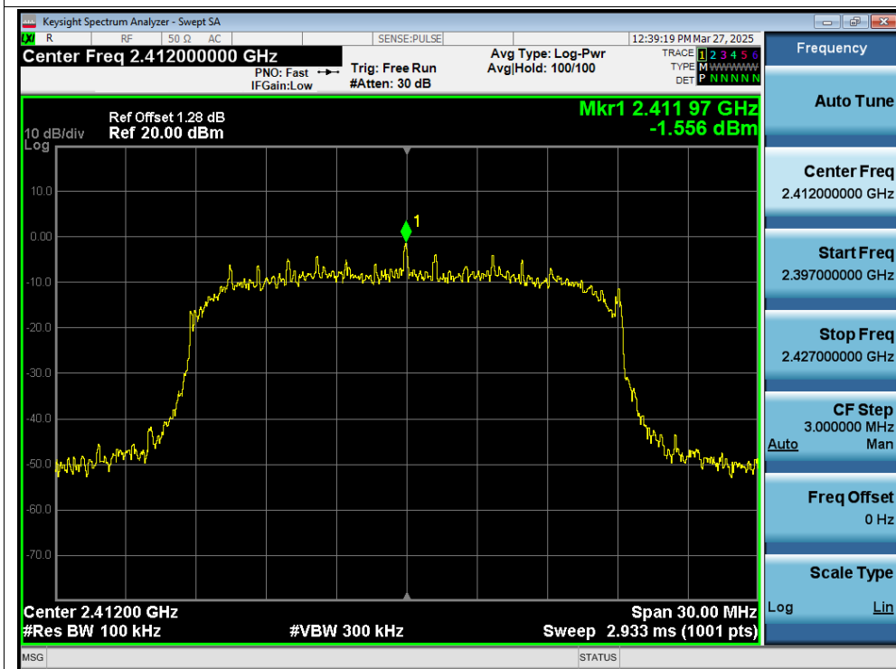
Band Edge NVNT n20 2412MHz Ant1 Emission
