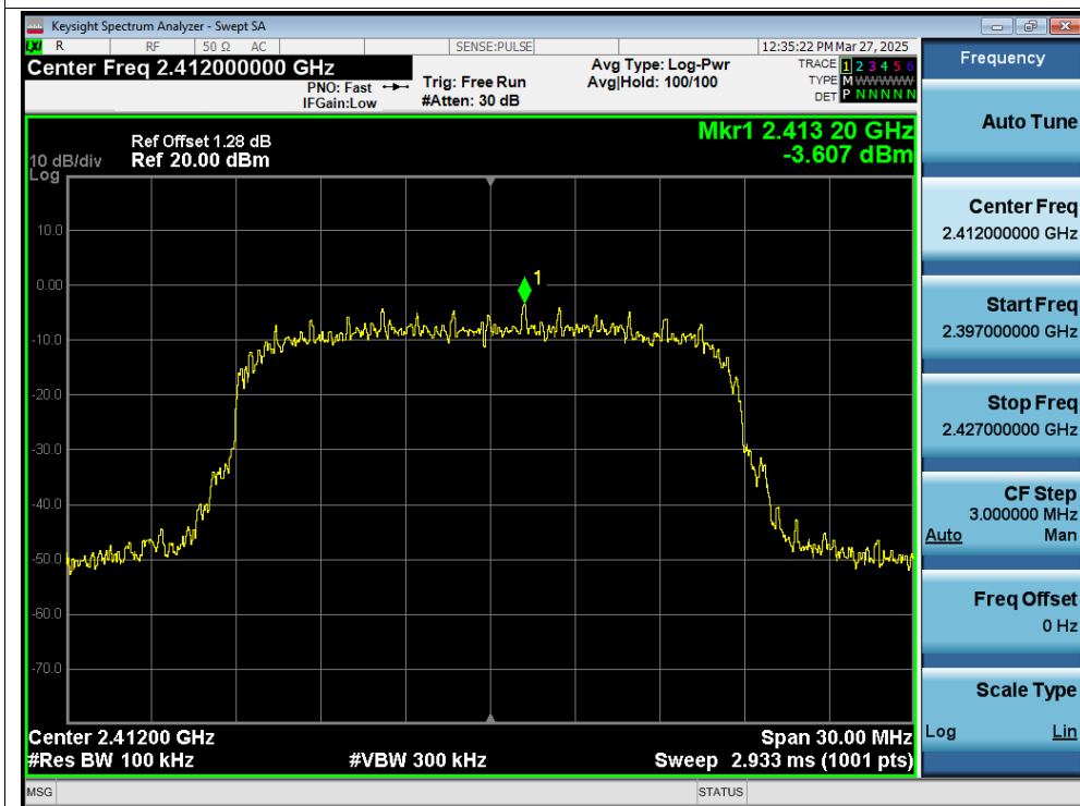
Band Edge NVNT g 2412MHz Ant1 Emission
