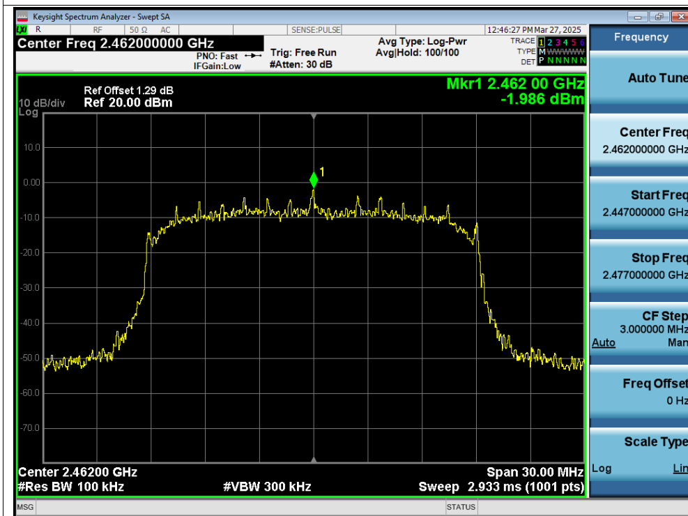
Tx. Spurious NVNT n20 2462MHz Ant1 Emission
