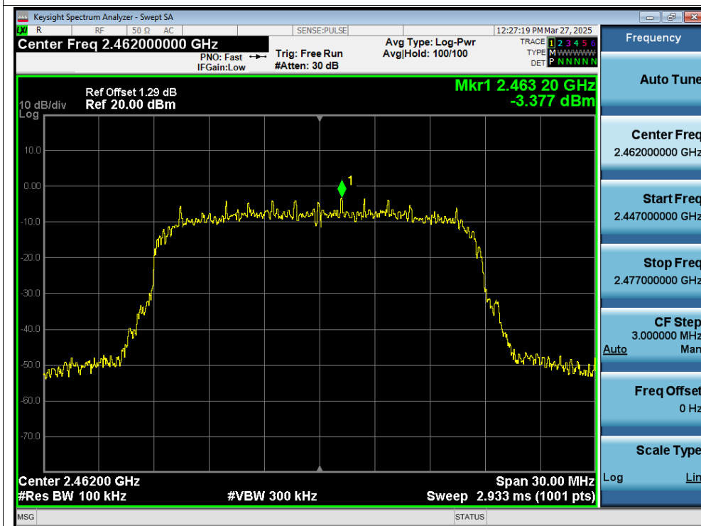
Tx. Spurious NVNT g 2462MHz Ant1 Emission
