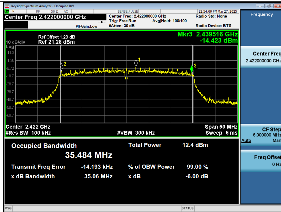
-6dB Bandwidth NVNT n40 2422MHz Ant1
